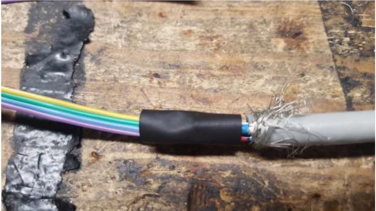
87) Apply heat to the 1/4" heatshrink to insulate the bundle of soldered wires.
